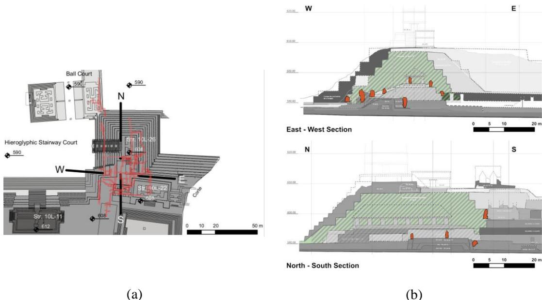
Figure 13. (a) Detail of the Acropolis plan showing the extension of currently open tunnels under the Hieroglyphic Stairway Temple (in red) – adapted from PAAC drawings; (b) Sections of the Hieroglyphic Stairway Temple showing the approximate positions of tunnels (in red) and the green hatch of the Esmeralda volume – adapted from C. Rudy Larios' PAAC drawings (modified after Pires *et al.*, 2021).
