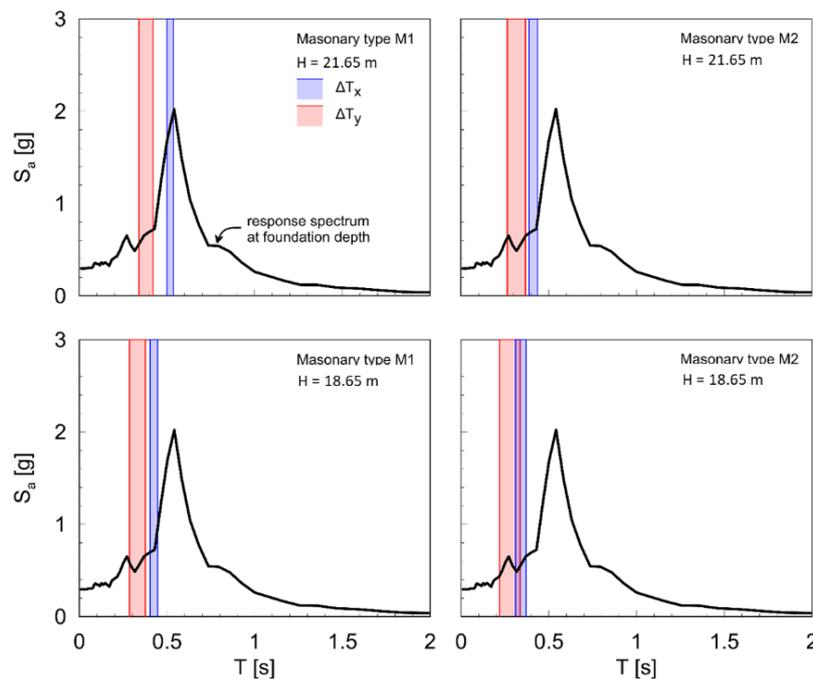
Figure 46. Equivalent elastic analyses: tower 19 seismic demand considering or neglecting dynamic soil-structure interaction in the two directions  $x$  and  $y$ , for both types of masonries (M1 and M2) and for different ways to consider the height of the mass centroid: at the foundation level ( $H=21.65$  m) or at ground level ( $H=18,65$ ). Period elongation indicated by the coloured bands (see legend on top left) (modified after Somma et al., 2022).
