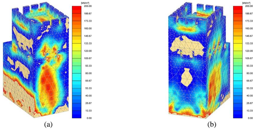
Figure 48. (a) Contours of the principal maximum tensile stresses in the laterally disconnected tower in x-direction at 5.60 s; (b) Contours of the principal maximum tensile stresses in the laterally disconnected tower in y-direction at 7.05 s.
