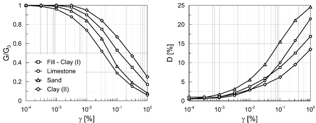
Figure 42. Shear modulus and damping ratio curves for the different soil layers (modified after Flora *et al.*, 2021).
