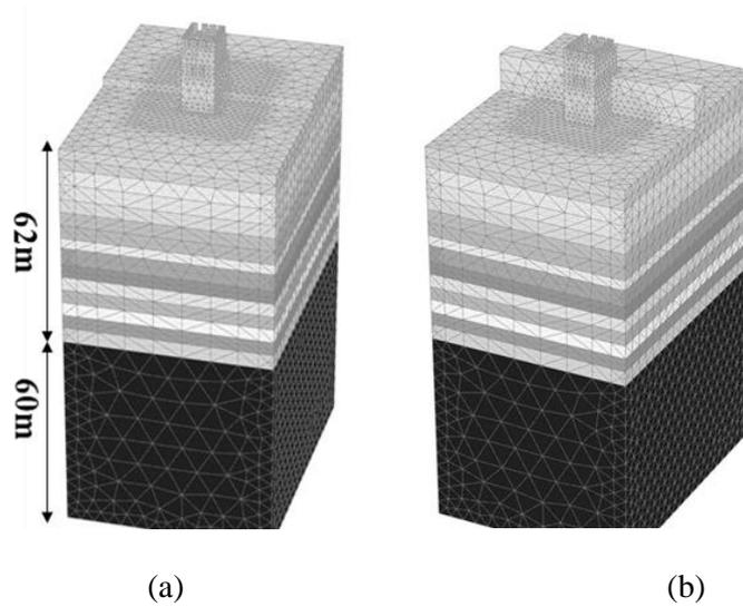
Figure 45. Plaxis3D model of the subsoil with Tower 19 considering (a) or neglecting (b) the inner wall.
