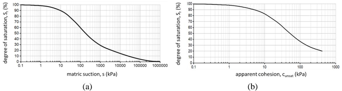
Figure 21. (a) Soil-water characteristic curve and (b) apparent cohesion versus saturation, for the silty sand infill (*girún*).
