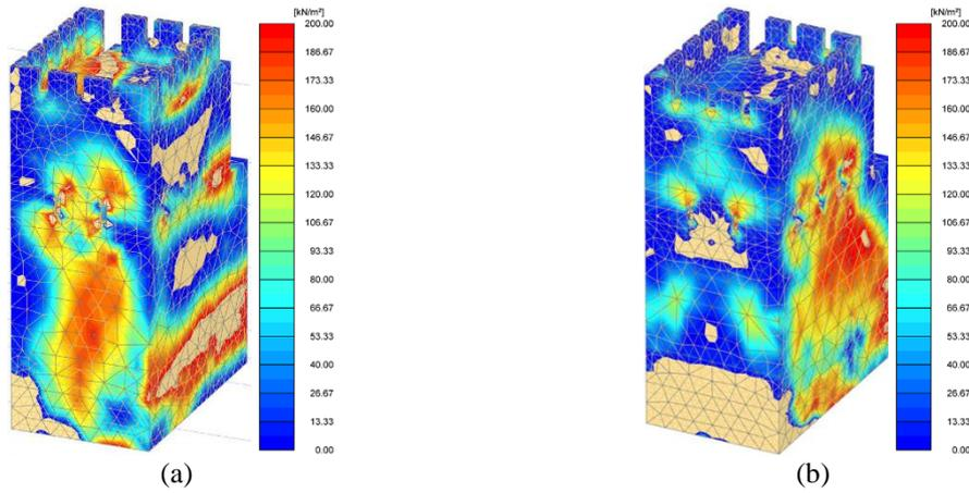
Figure 47. (a) Contours of principal maximum tensile stresses for tower 19 (compliant base, masonry M1): (a) seismic action in the x direction; (b) seismic action in the y direction.
