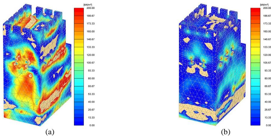
Figure 49. (a) Contours of the principal maximum tensile stresses in the laterally stiffened tower in x-direction at 7.92 s; (b) Contours of the principal maximum tensile stresses in the laterally stiffened tower in y-direction at 6.72 s.
