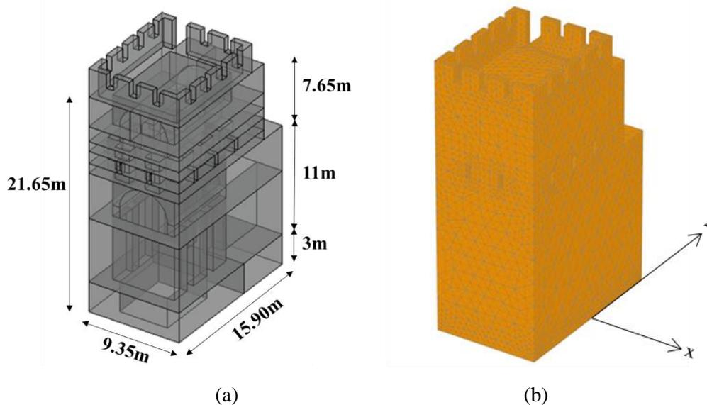
Figure 44. Tower 19: (a) geometric model and (b) Plaxis3D mesh ( $x$ =wall's longitudinal axis;  $y$ =wall's transversal axis).
